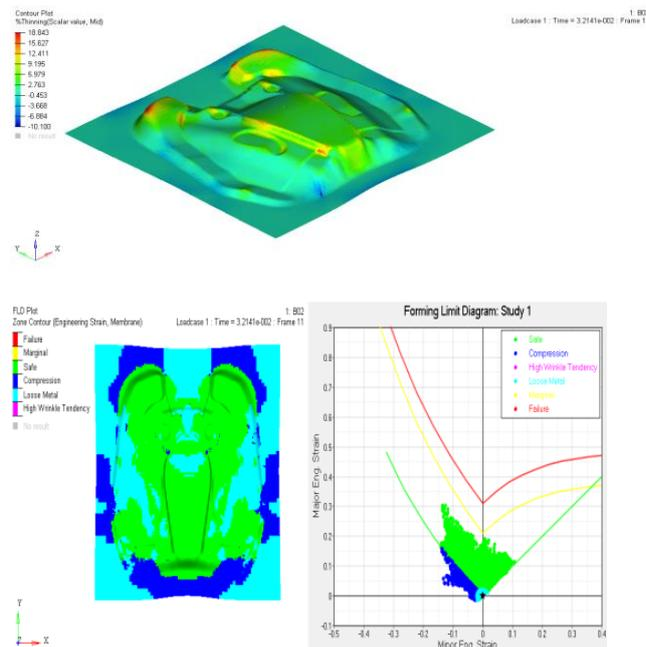
Figure 8: Simulation result of 1<sup>st</sup> iteration
