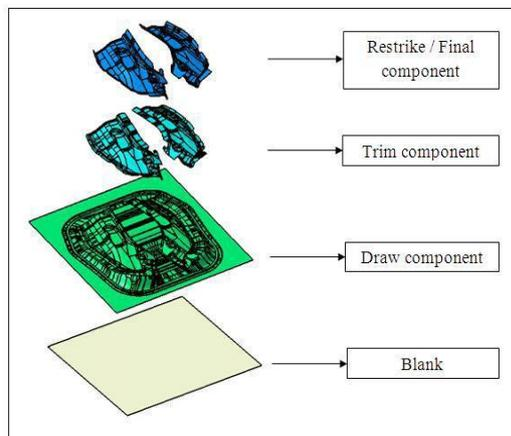
**Figure 4:** The complete process to manufacture REINF-RR END UPR-LH/RH
