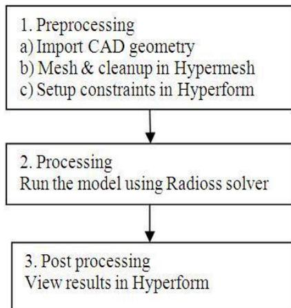
**Figure 6:** Steps in the simulation process
