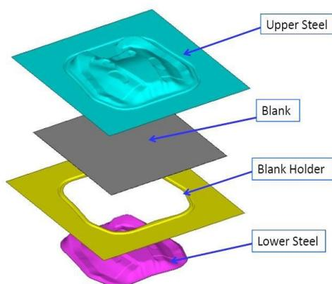
**Figure 7:** Forming tool set up
