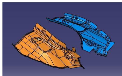
Figure 3: CAD model of REINF-RR END UPR-LH/RH
