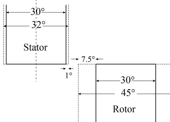
Fig.12: Rotor & stator pole arc
