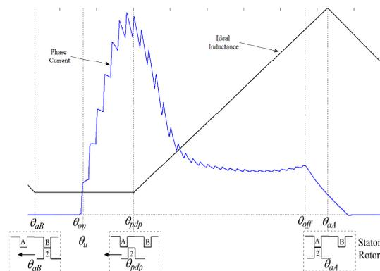
**Fig.1:** Phase current and phase inductance for voltage PWM controlled drive
