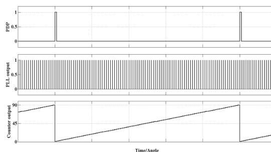
Fig.9: Output of pulse counter
