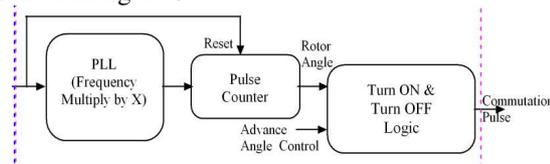
Fig.6: Commutation logic block
