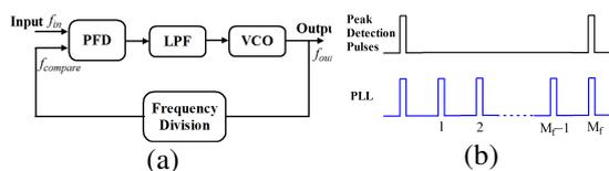
Fig.7: (a) PLL block diagram (b) Output of PLL
