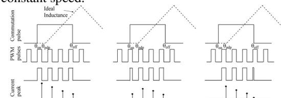
Fig.13: PWM pulse, commutation pulse and current
