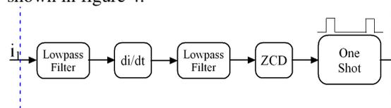
Fig.3: Current peak detection block
