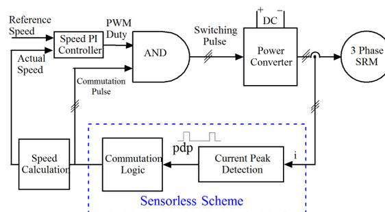
Fig.5: PWM controlled sensorless drive with CGSM
