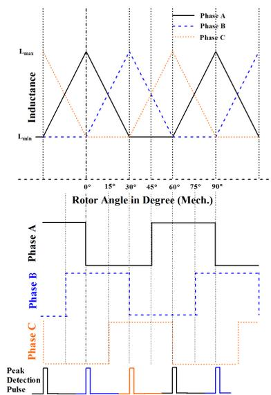
Fig.8: Peak detection pulse for each Phase
