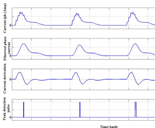
Fig.4: Output waveform at each stage of current peak detection
