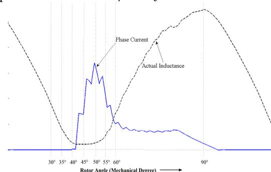
Fig.11: Phase current and inductance variation of 60KW, 6/4 pole, 3 phase SRM
