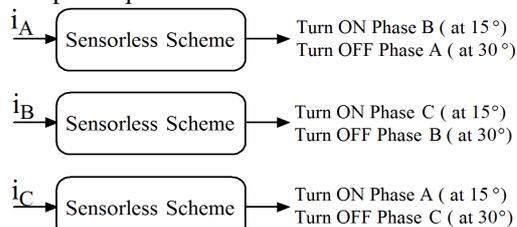
Fig.10: Phase commutation logic
