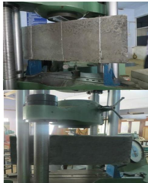
**Fig. 4 Three point bending test on beam**
