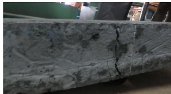
Fig. 9 Crack pattern – Bottom view
