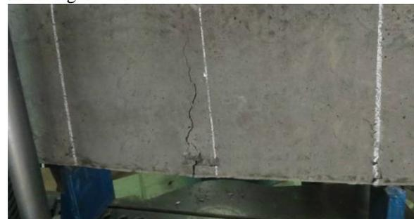
Fig. 8 Crack pattern – Front view
