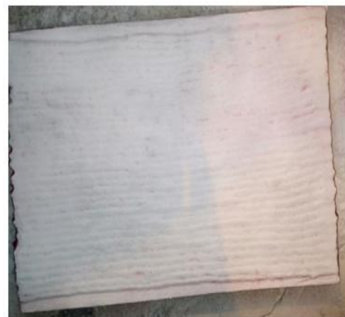
Fig.5 Dye Penetrate examination
