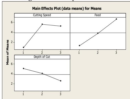
From Table 9, it is clear that feed is the most influencing factor followed by cutting speed and depth of cut for surface roughness. The optimum value for surface roughness is predicted from Fig 6, i.e. cutting speed of 384 rpm, feed of 0.0625 mm/rev and depth of cut of 0.4 mm. From Fig 9 and 10 it is clear that the HSS tool is the most suitable tool for minimized surface roughness and maximized material removal rate with maximum speed when compared to Carbide and PCD tools.
