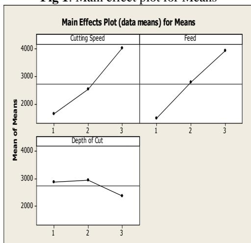
From Table 4, it is clear that feed is the most influencing factor followed by cutting speed and depth of cut for MRR. The optimum value for MRR is predicted from Fig 1, i.e. cutting speed of 938 rpm, feed of 0.1875 mm/rev and depth of cut of 0.3 mm.
