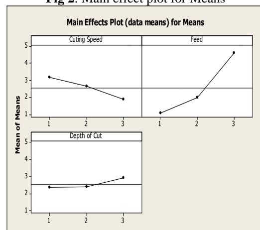
From Table 5, it is clear that feed is the most influencing factor followed by cutting speed and depth of cut for surface roughness. The optimum value for surface roughness is predicted from Fig 2, i.e. cutting speed of 938 rpm, feed of 0.0625 mm/rev and depth of cut of 0.2 mm.
