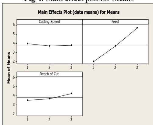
From Table 7, it is clear that feed is the most influencing factor followed by depth of cut and cutting speed for surface roughness. The optimum value for surface roughness is predicted from Fig4, i.e. cutting speed of 598 rpm, feed of 0.0625 mm/rev and depth of cut of 0.2 mm.
