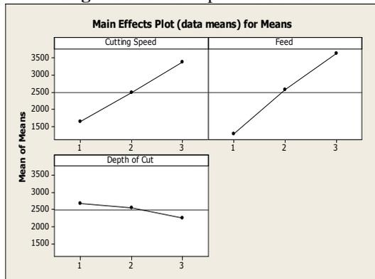
From Table 6, it is clear that feed is the most influencing factor followed by cutting speed and depth of cut for MRR. The optimum value for MRR is predicted from fig 3, i.e. cutting speed of 938 rpm, feed of 0.1875 mm/rev and depth of cut of 0.2 mm.
