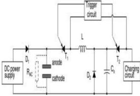
Fig. 2 Electrical circuit for pulse (spark) generation [9]
