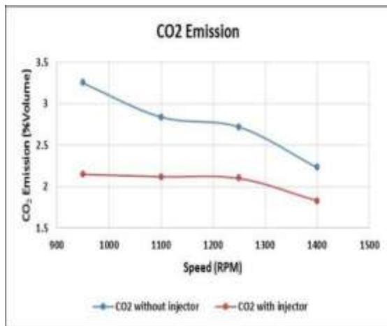
Fig 4.3: Speed v/s CO<sub>2</sub> Emission
