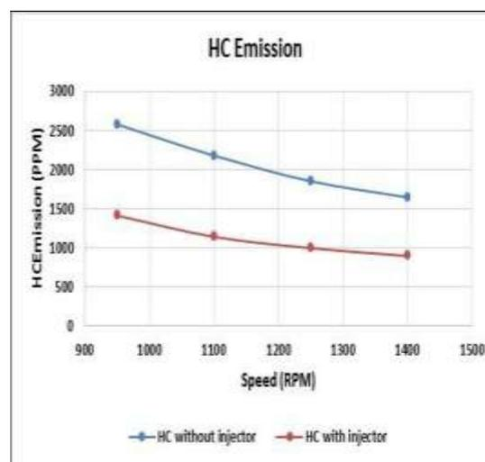
Fig 4.2: Speed v/s HC Emission
