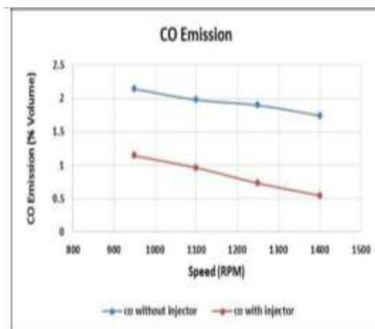
Fig 4.1: Speed v/s CO Emission
