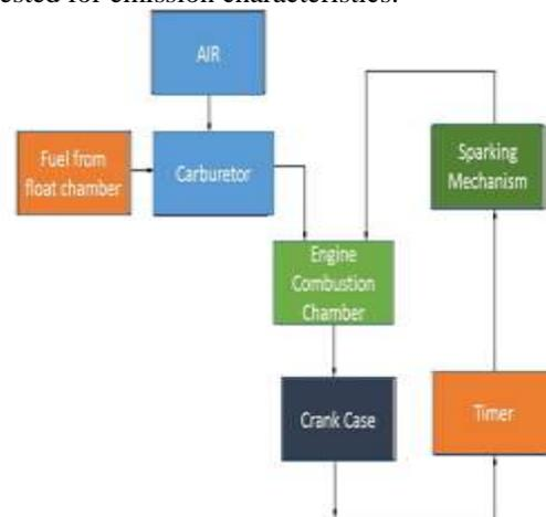
Fig 3.1: Block diagram of conventional two stroke
