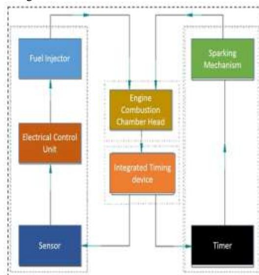
Fig 3.2: Block diagram of modified Two Stroke SI-Engine (DFI-System)
