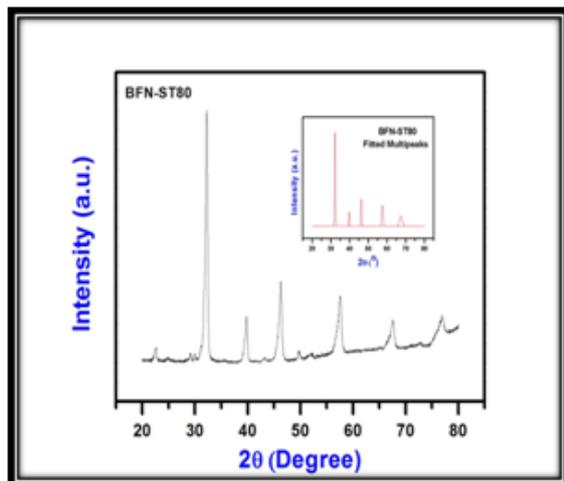
Figure 1. X-ray diffraction patterns of BFN-ST80 nanomaterials , at room temperature.
