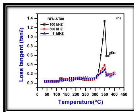
Figure 6(a)-(b) Shows variation of loss tangent with temperature in BFN-ST80 nanoceramic for different frequency ranges
