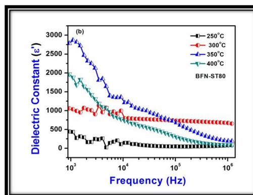
Figure 3 (a) and (b) shows Frequency dependence behavior of real part of Dielectric Constant at different temperatures.
