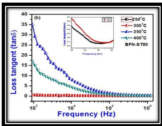
Figure 4 (a) and (b) shows Frequency dependent loss tangent at different temperatures.
