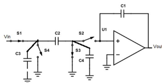
Fig.5 SC parasitic insensitive or classical integrator
