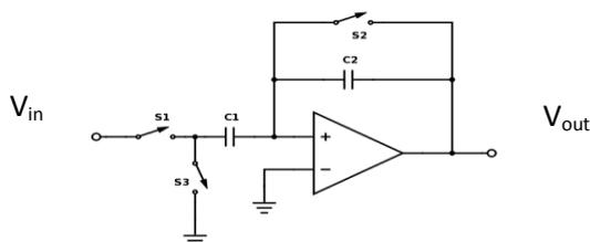
Fig. 1 Switched-capacitor amplifier
