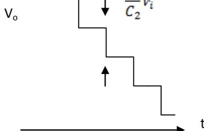
Fig. 4 Staircase resultant of Switched-Capacitor Integrator
