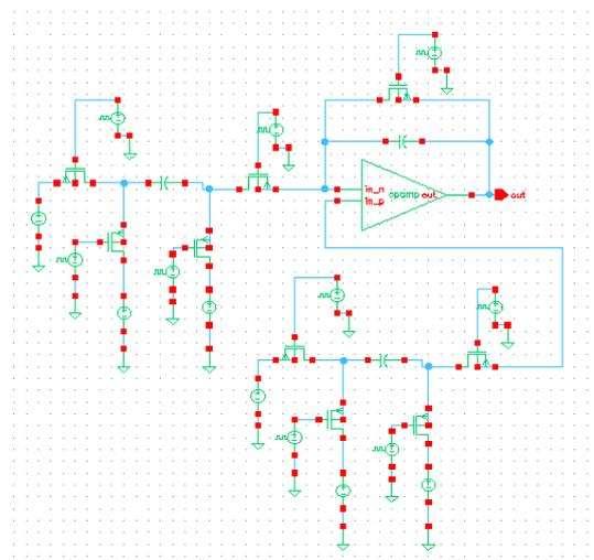
Fig.7 Schematic diagram of Modified SC integrator
