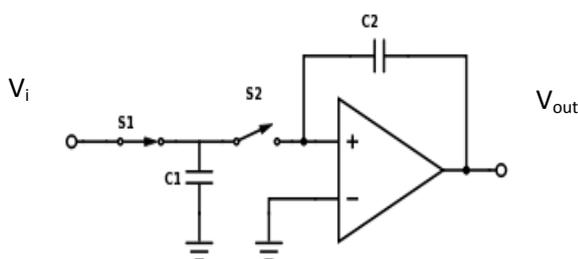
Fig. 3 Fundamental Switched-Capacitor Integrator
