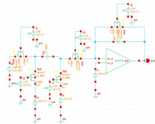
Fig.6 Schematic diagram of SC integrator
