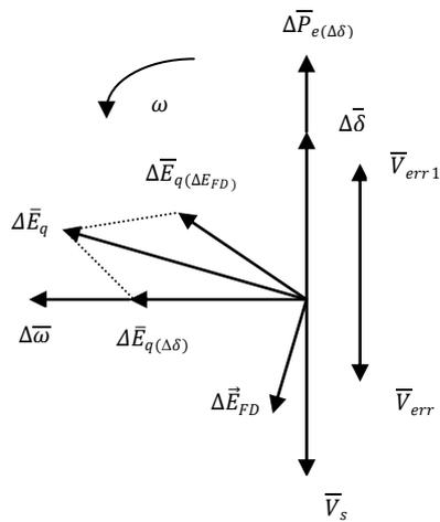
Figure 2 Phasor diagram of the PSS application [11]
