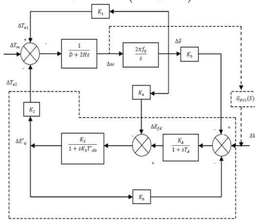
**Figure 4** PSS with Heffron-Philips model of a single-machine infinite-bus system
