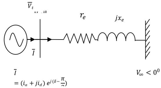
Figure 3 System of a synchronous machine connected to an infinite bus or SMIB [9]
