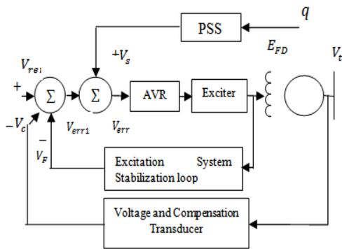
Figure 1 Block diagram of the PSS application [11]
