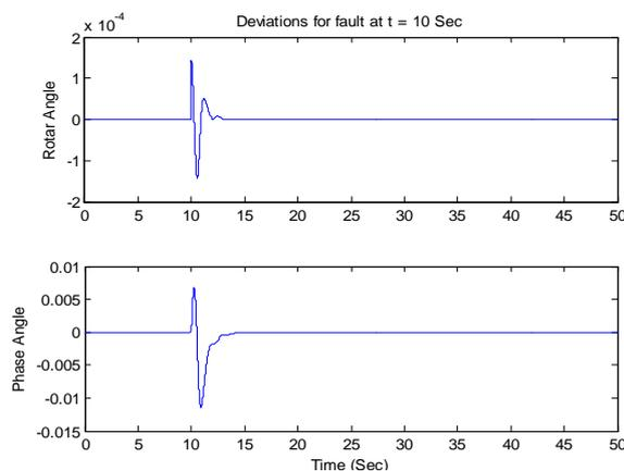
**Figure 6** Rotor angle and phase angle deviations in SMIB-PSS optimized with ABC Algorithm
