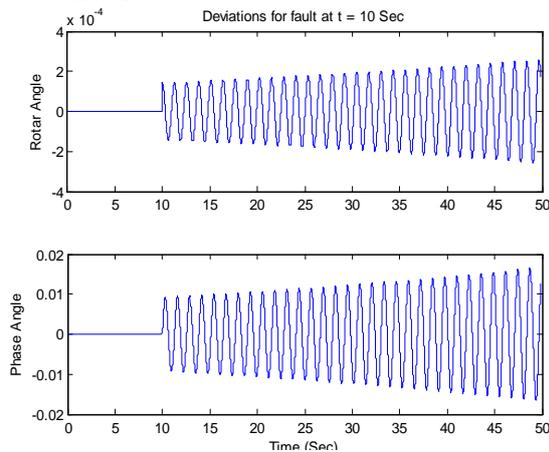
**Figure 5** Rotor angle and phase angle deviations in SMIB-PSS without optimization
