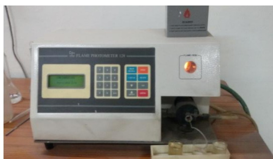
Fig.2. Determination of Sodium and Potassium using Flame Photometer.
