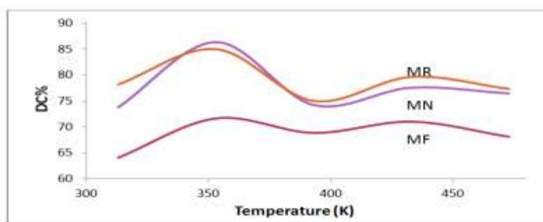
**Fig . 2** – Variation of degree of crystallinity of muga fiber with temperature. ( MR- Muga raw, MN- Muga degummed by Na<sub>2</sub>CO<sub>3</sub>, MF- Muga degummed by formaldehyde)
