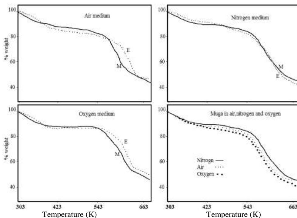
**Fig.6.** TG thermograms of raw muga fibers in air, oxygen and air medium.
