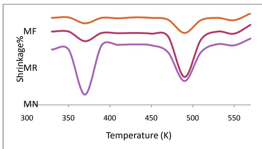
**Fig.4-** Dry heat shrinkage of raw and degummed muga fibers with temperature.
