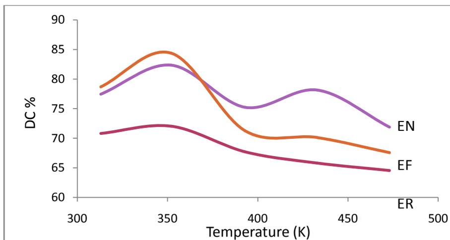
**Fig. 3-** Variation of degree of crystallinity of eri fiber with temperature.
