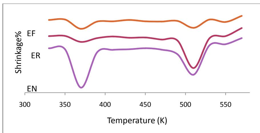
**Fig.5-** Dry heat shrinkage of raw and degummed eri fibers with temperature.
