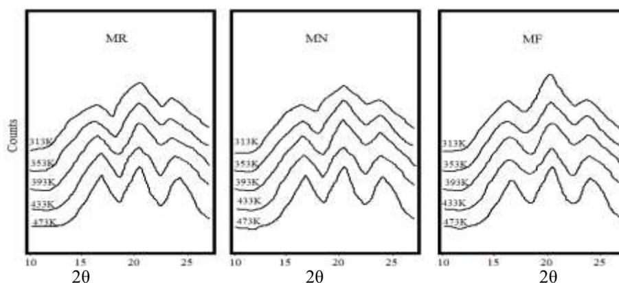
Fig.1- XRD of raw and degummed muga fiber at different temperatures.
