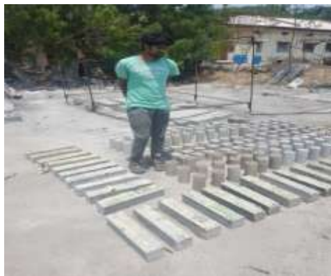
Figure 6.0 Specimens curing in Ambient Temperature.
