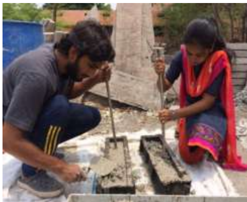
Figure 5.0 Prism specimens casted
