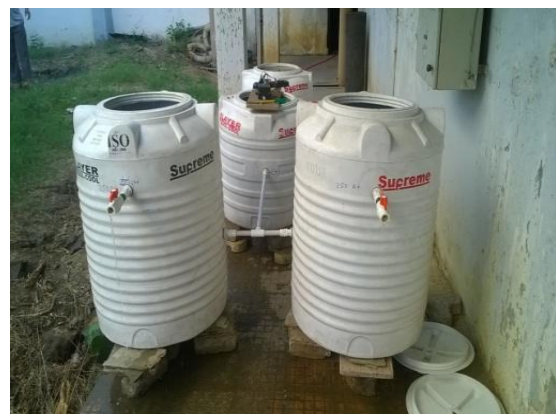
Fig. Setup for Backwash water treatment
