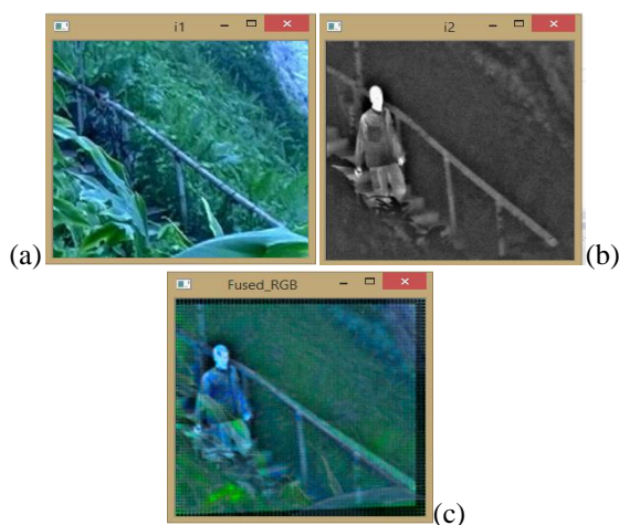
Fig 7 Image Fusion for Still Images (a) EO image, (b) IR image, (c) Fused Image
