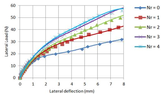
Fig. 8: Load Deflection Curve for Long Pile at  $b=2.5D$  and  $\theta=30^\circ$
