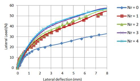
**Fig. 4:** Load Deflection Curve for Long Pile at b=7.5D and  $\theta=0^\circ$
