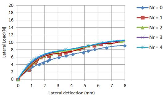
Fig. 13: Load Deflection Curve for Short Pile at  $b=7.5D$  and  $\theta=0^\circ$
