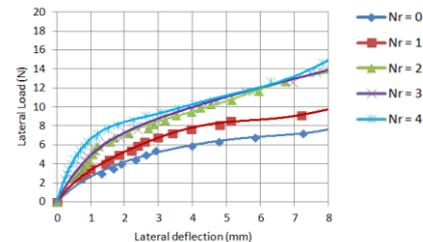
Fig. 15: Load Deflection Curve for Short Pile at  $b=5D$  and  $\theta=15^\circ$
