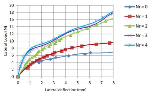
Fig. 17: Load Deflection Curve for Short Pile at  $b=2.5D$  and  $\theta=30^\circ$
