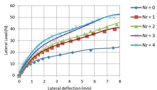
**Fig. 3:** Load Deflection Curve for Long Pile at b=5D and  $\theta=0^\circ$
