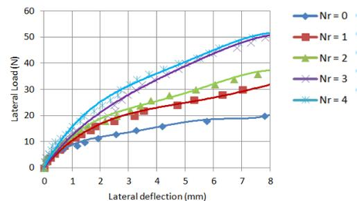
**Fig. 2:** Load Deflection Curve for Long Pile at b=2.5D and  $\theta=0^\circ$
