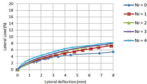
Fig. 11: Load Deflection Curve for Short Pile at  $b=2.5D$  and  $\theta=0^\circ$
