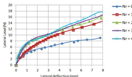
Fig. 16: Load Deflection Curve for Short Pile at  $b=7.5D$  and  $\theta=15^\circ$
