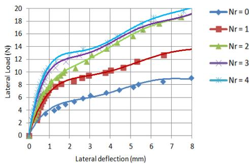
**Fig. 18:** Load Deflection Curve for Short Pile at  $b=5D$  and  $\theta=30^\circ$
