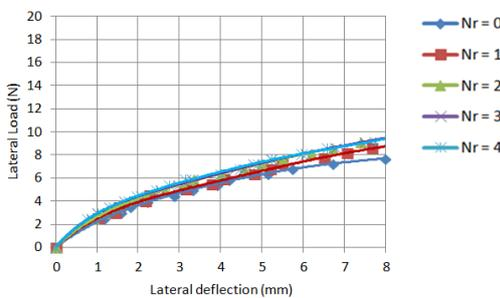
Fig. 12: Load Deflection Curve for Short Pile at  $b=5D$  and  $\theta=0^\circ$
