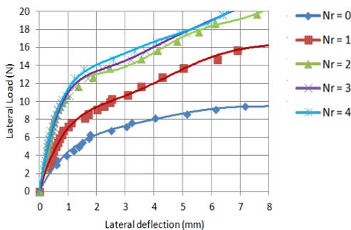
**Fig. 19:** Load Deflection Curve for Short Pile at  $b=7.5D$  and  $\theta=30^\circ$
