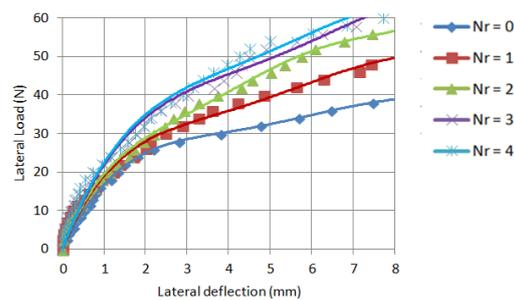
Fig. 9: Load Deflection Curve for Long Pile at  $b=5D$  and  $\theta=30^\circ$
