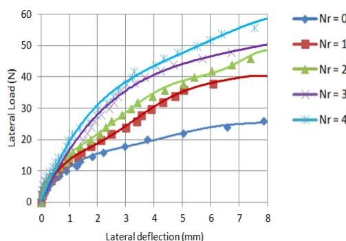
Fig. 6: Load Deflection Curve for Long Pile at  $b=5D$  and  $\theta=15^\circ$
