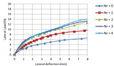
Fig. 14: Load Deflection Curve for Short Pile at  $b=2.5D$  and  $\theta=15^\circ$
