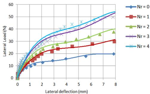
Fig. 5: Load Deflection Curve for Long Pile at  $b=2.5D$  and  $\theta=15^\circ$
