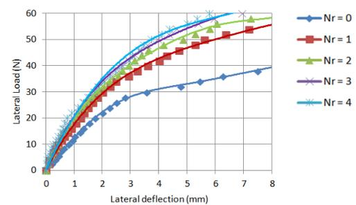
Fig. 10: Load Deflection Curve for Long Pile at  $b=7.5D$  and  $\theta=30^\circ$
