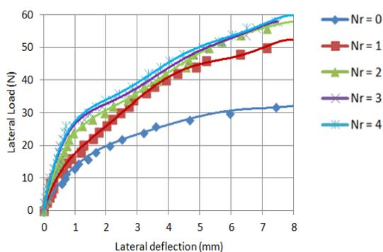
Fig. 7: Load Deflection Curve for Long Pile at  $b=7.5D$  and  $\theta=15^\circ$
