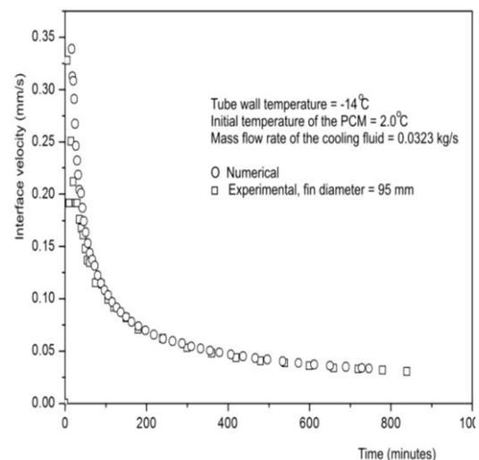
**Figure 3** Numerical and experimental comparison of the instantaneous interface velocity for a finned tube of 95 mm diameter.
