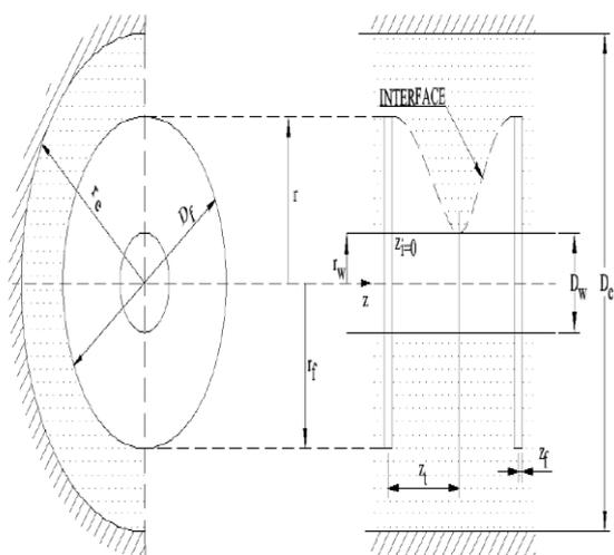
**Figure 1** Sketch of the problem of phase change around a finned tube.
