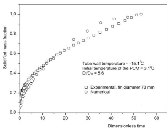
**Figure 6** Numerical and experimental comparison of the solidified mass fraction for a finned tube of 70 mm diameter.
