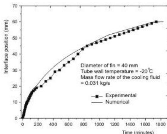
**Figure 7** Numerical and experimental comparison of the radial interface position for a finned tube of 40 mm diameter.
