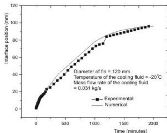
**Figure 8** Numerical and experimental comparison of the radial interface position for a finned tube of 120 mm diameter.
