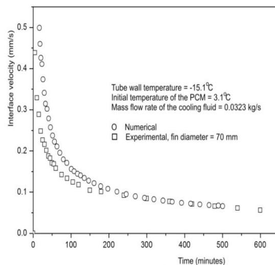
**Figure 4** Numerical and experimental comparison of the instantaneous interface velocity for a finned tube of 70 mm diameter.
