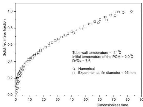
**Figure 5** Numerical and experimental comparison of the solidified mass fraction for a finned tube of 95 mm diameter.
