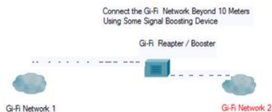
Figure 11: proposed Gi-Fi network with repeaters
