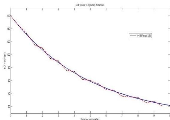
Figure2: RSSI distribution against distance between a transmitter and a receiver
