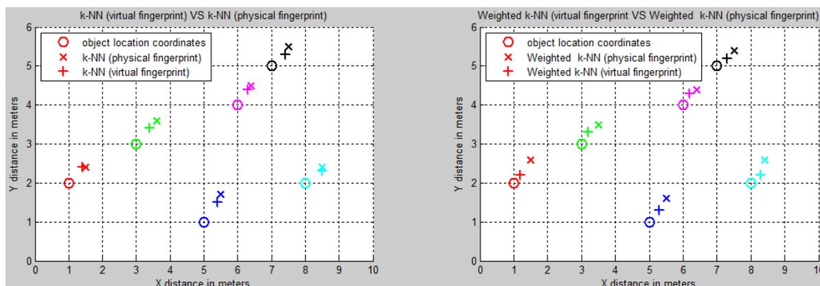
**Figure 5:** Localization with virtual and physical fingerprinting with adaptive correction
