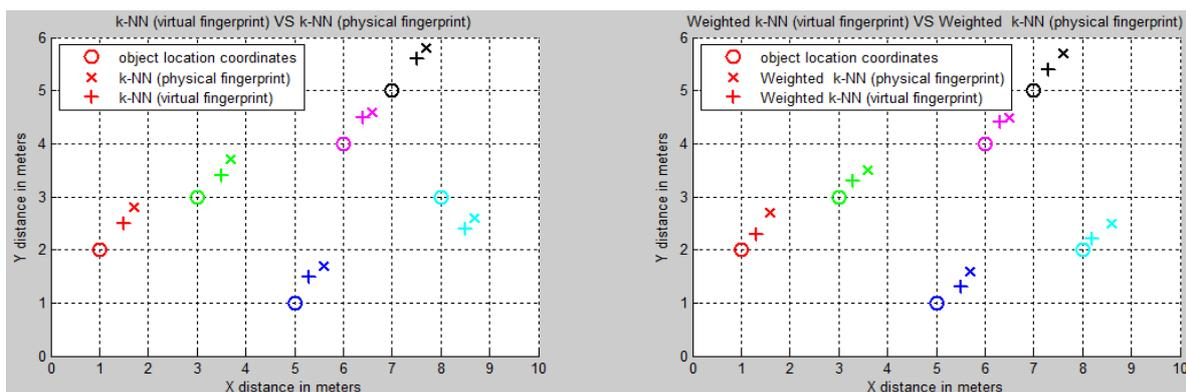
**Figure 4:** localization with virtual and physical fingerprinting with no adaptive correction
