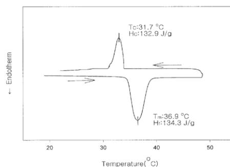
**Fig. 2** DSC thermogram of the microcapsules
