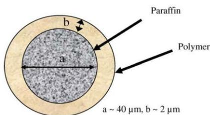
**Fig. 1** Microencapsulation: Paraffinic PCM core material individually with a hard polymeric shell
