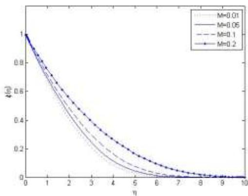
Fig.4: Concentration profiles for different values of  $M$
