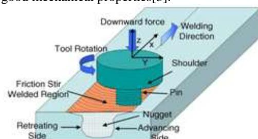
Fig. 1 Friction stir welding process [2]
