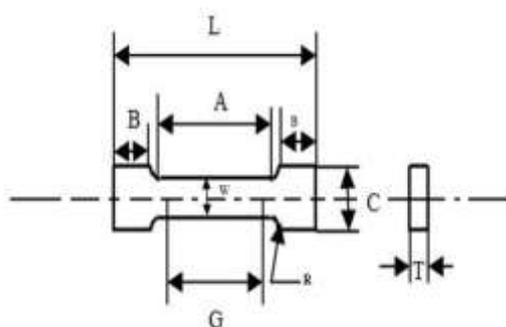
Fig. 6 Tensile test specimen diagram
