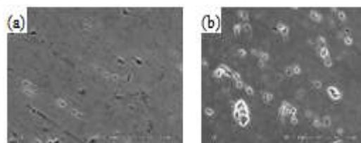
Fig. 16 Microstructure of parent material (a) AL6101T6 and (b) AL6351T6
