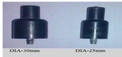
Fig. 3 FSW tools with threaded tip
