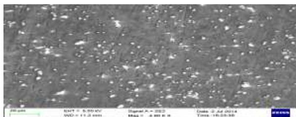
Fig.18(b) Oxide layer formation in Weld centre
