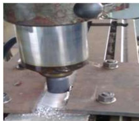
Fig. 4 FSW experimental Set-up
