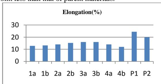
Fig 10: % Elongation of base metal and welds
