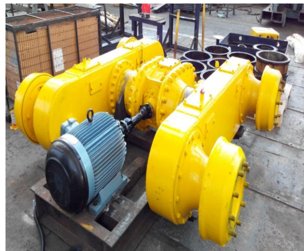
Figure 9: Interfacing of motor and tandem jig
