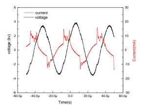
Fig.3: Voltage and current waveforms of discharge.
