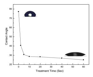
Fig 5: Water contact angle on PET as function of treatment time in Argon plasma
