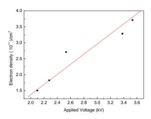
Fig 4: Electron density as a function of applied voltage.
