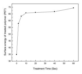
Fig 6: Surface energy of PET as function of treatment time in Argon plasma
