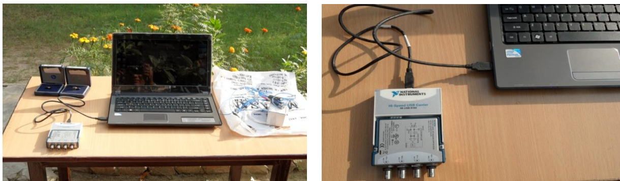
Figure 2 : The items used in data acquisition process (Triaxil transducer, Adaptor to hold transducer, data acquisition card and interfacing with Laptop)
