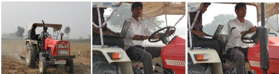
Figure 3 : (a) FARMTRAC 50 model on ploughing field , (b)Sensors position on steering and lower arm (wrist), (c) Sensors position on steering and upper arm
