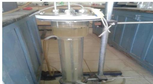
Fig: Fluidised Bed Reactor
