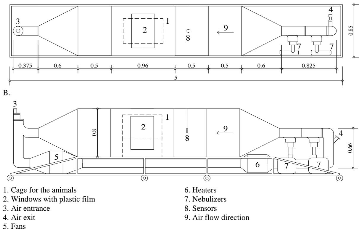
Figure 2. Top (a) and lateral (b) views of the wind tunnel
