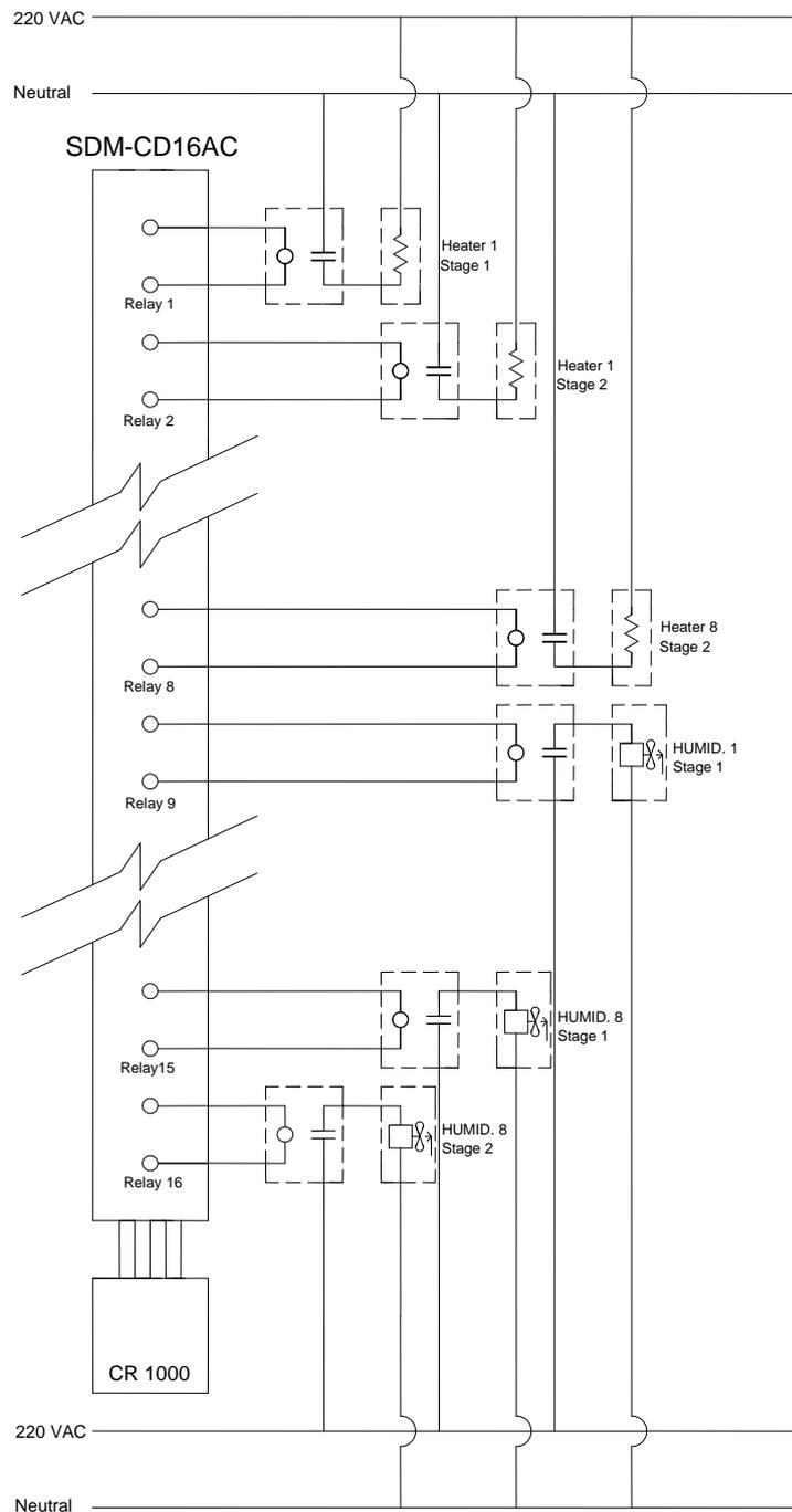
Figure 3. Simplified scheme representing the electric circuit for  $t_{air}$  and RH control inside the wind tunnels
