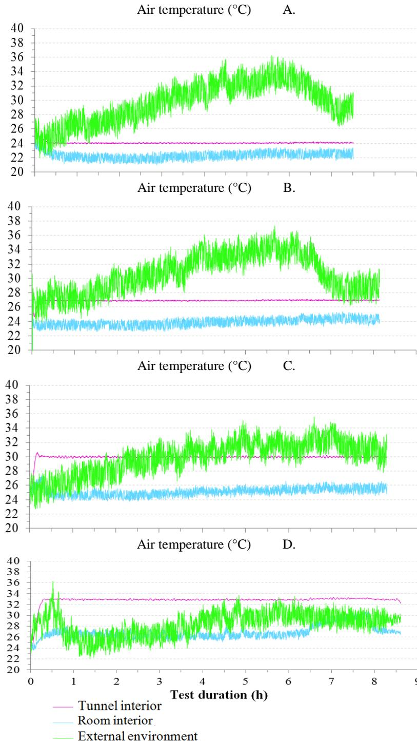
Figure 7. Behavior of the air temperature inside the wind tunnel, inside the room and in the external environment for the set points at 24 (a), 27 (b), 30 (c) and 33 °C (d)
