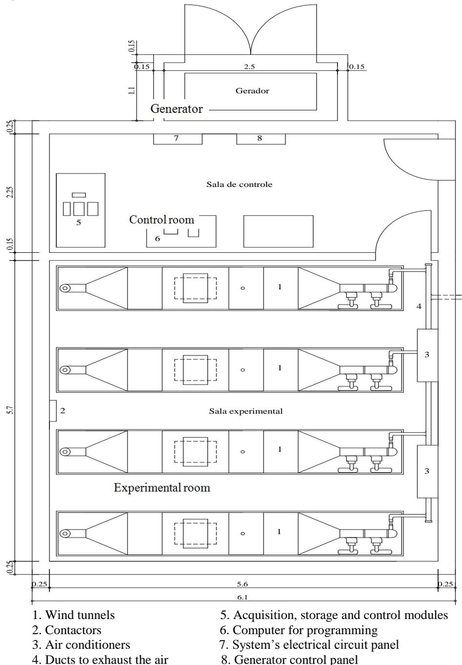
Figure 1. Illustrative scheme of the wind tunnels installed inside a room equipped with system cooling
