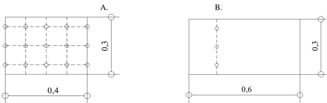
Figure 5. Representation of the measurement points for air velocity in the transversal (a) and longitudinal (b) sessions of the cage
