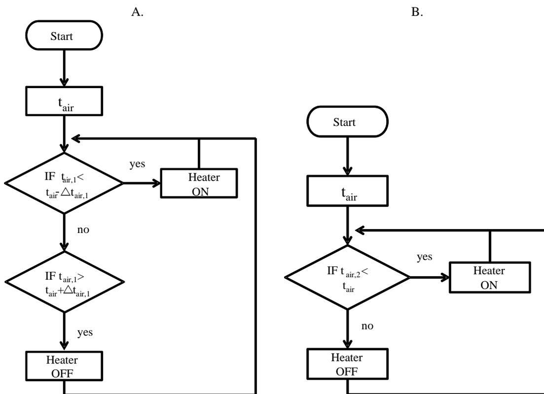
Figure 4. Flowchart illustrating the logic of  $t_{air}$  control for the stages 1 (a) and 2 (b). The same logic is applied to RH control
