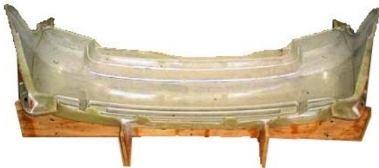
Figure 06: Mold of the rear bumper in real scale.
