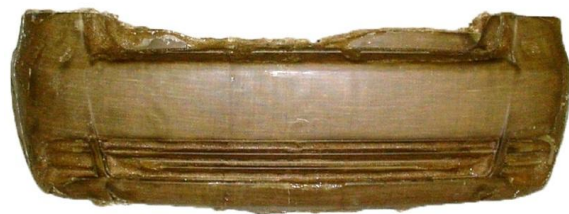
Figure 08: External surface of orthohtalic polyester resin and fiber of jute Bumper.
