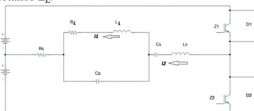
Fig.4. (a) simplified circuit of the inverter system
