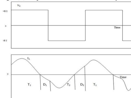
Fig.4. (b) typical steady state waveforms of the inverter output voltage  $v_o$  and current  $i_1$  at a leading power factor
