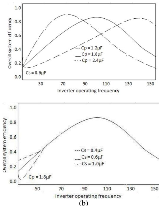
Fig.5. (a) Calculated current gain as a function of the inverter operating frequency with  $C_s$  and  $C_p$  parameters ( $E = 40$  V). (b) Overall system efficiency versus the inverter operating frequency with  $C_s$  and  $C_p$  parameters ( $E = 40$  V)
