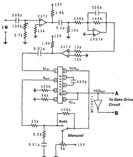
Fig. 2.Phase-locked loop (PLL) control circuit.
