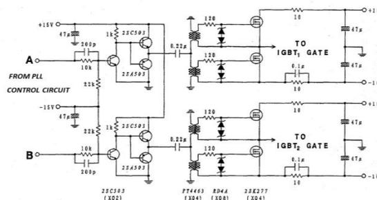
Fig.3. IGBT drive circuit.
