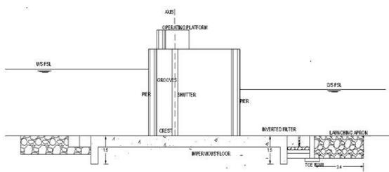
Fig. 6 Longitudinal cross section of Regulator
