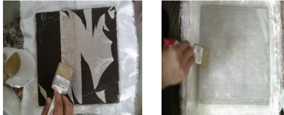
Figure 4: Bonding of Glass Fabric to the Core
