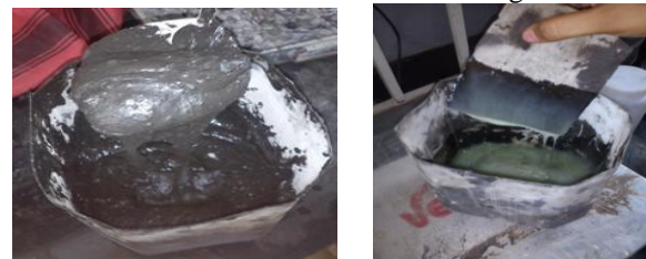
Figure 2: Mixing of Measured Fly Ash, Resin and Hardener
