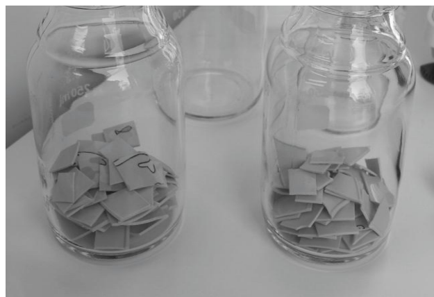
Figure 2.1 Plastic product (bib for babies), and synthetic textiles (sporting sweater, stretch pants, and knitted muffler), prior to leaching.
