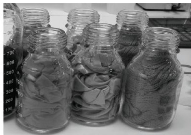
Figure 2.1 Synthetic Textiles (Sporting Sweater, Stretch Pants, And Knitted Muffler), Prior To Leaching.
