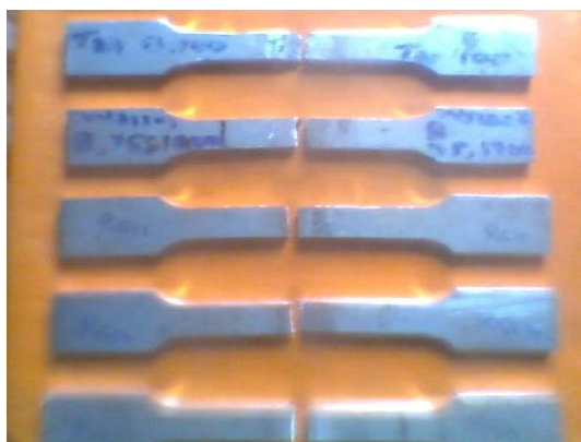
Figure .8 Tensile test specimens of Friction Stir Welded joints of AA7075 after.
