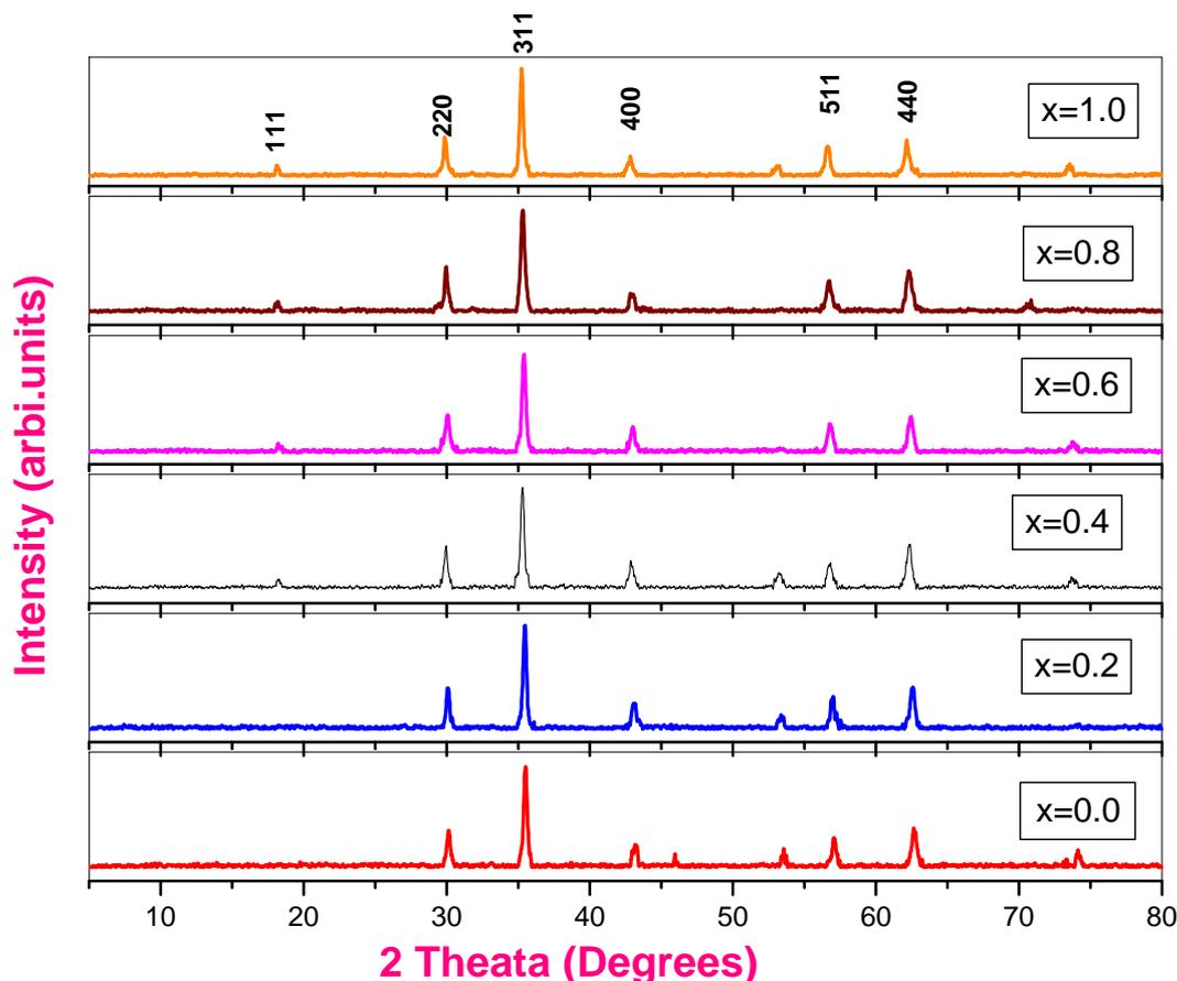
Figure 1.XRD patterns of  $Mg_{1-x}Zn_xFe_2O_4$  nano ferrites
