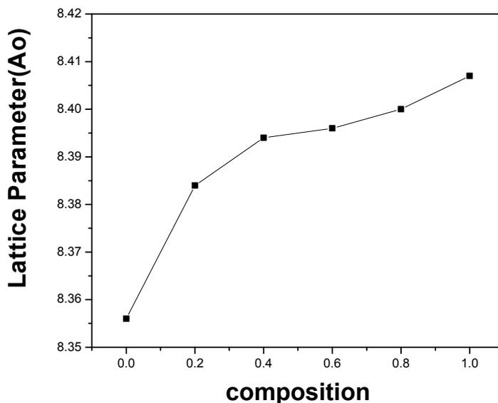
**Figure2. Variation of lattice parameter with composition for Mg-Zn nano-ferrites**
