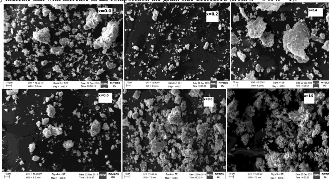
Figure5 SEM Diagrams of Mg-Zn Nano Ferrites
