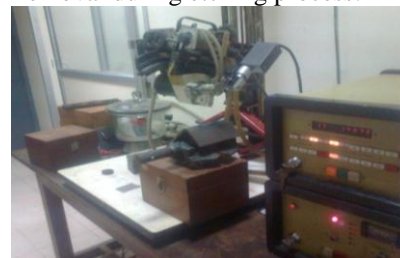
Fig. 13 X-ray diffraction measurement setup (Courtesy: Central X-ray diffraction lab, IIT Madras, India)
