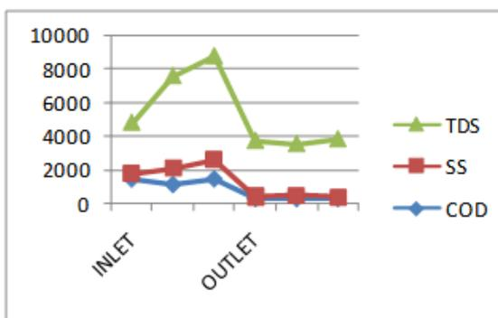
fig 3 COD, TDS and SS Removal Efficiency(after modification)
