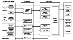
Figure 6. Autopilot and Guidance Flight Mode
