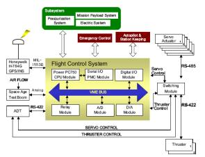
Figure 1. Autonomous Flight Control System
