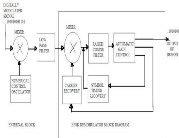
Fig II.3.BPSK Demodulator Block diagram
