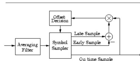
Figure 6: DLL block diagram.
