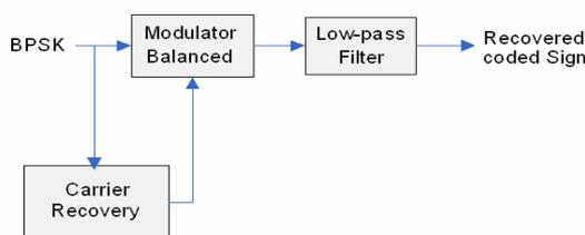
Figure I.3: Generic BPSK Demodulator Block Diagram.
