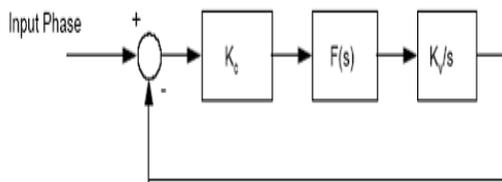
Figure 2: BPSK Costas Equivalent Loop Model
