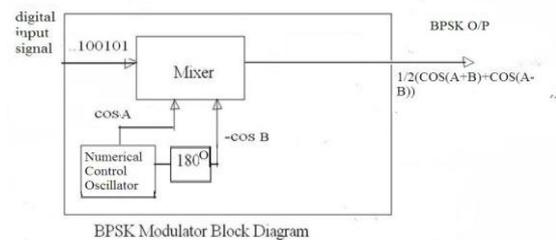
Fig.II.1.BPSK Modulator block diagram.
