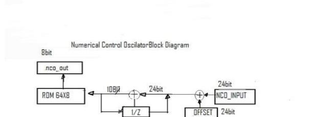
Fig.II.6.NCO oscillator block diagram
