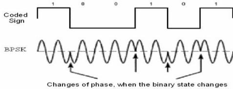
Figure 1.2: BPSK Modulation.
