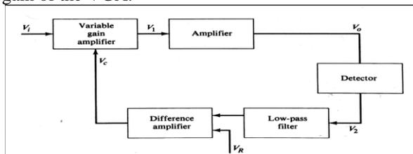
Fig.II.10. AGC block diagram
