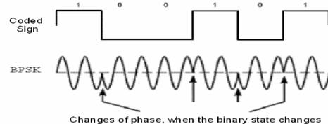
Fig.II.2.BPSK Modulation wave form.
