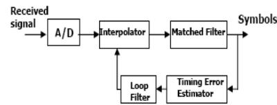
FigII.15: Digital filter timing recovery loop
