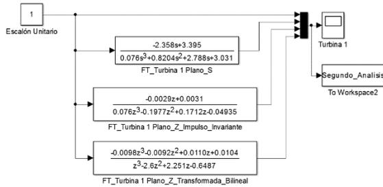
Fig. 4. Transfer Functions on Simulink with rounding.
