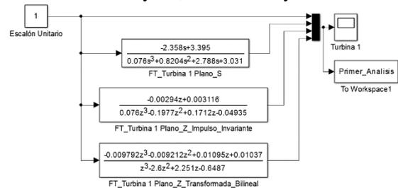
Fig. 2. Transference Functions on Simulink
