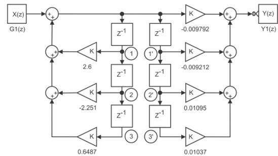
Fig. 7. Direct Structure Transpose I
