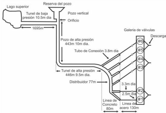
Fig. 1. Schematic diagram of the hydroelectric station (not on scale)
