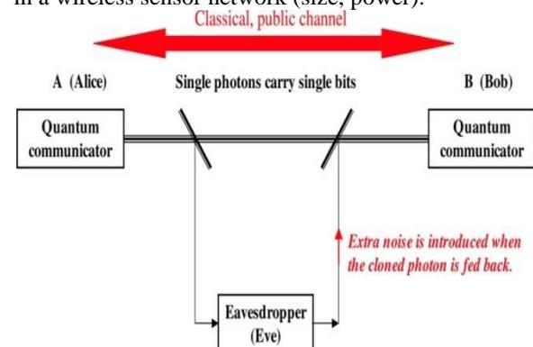
Fig.1:secure communication system
