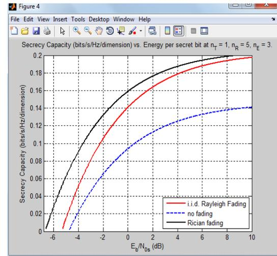
Fig.6: Comparison of different fading channels with no fading channel
