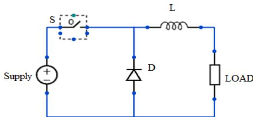
Fig.1. Buck converter circuit diagram
