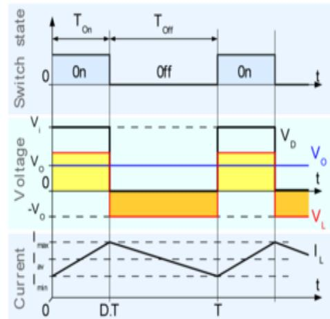
Fig.3: Evolution of the voltages and currents with time in an ideal buck converter operating in continuous mode.
