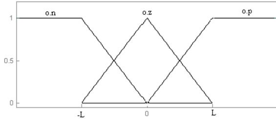
Fig.8 The membership functions of e(nT), r(nT) and u(nT).
