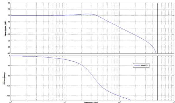
Fig 11 Magnitude and phase response of  $G_{vd}(Z)$  for digitally controlled buck converter with no losses
