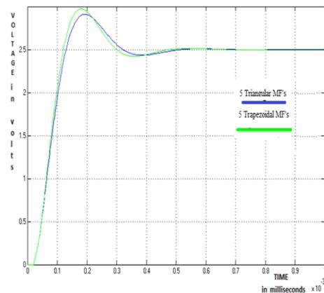
Fig. 13 Simulation of Buck Converter using triangular and trapezoidal five membership functions.
