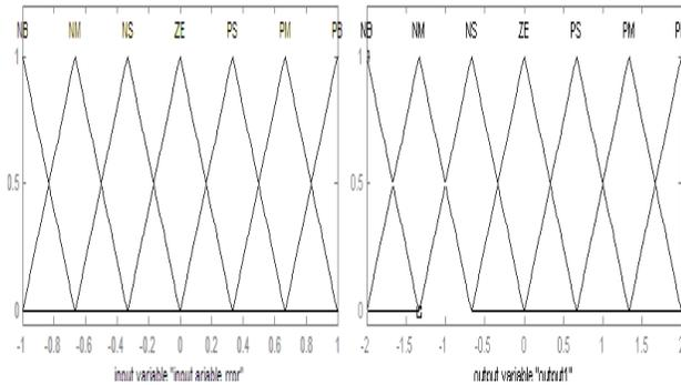
Fig.10 Triangular 7 membership functions of the error, output
