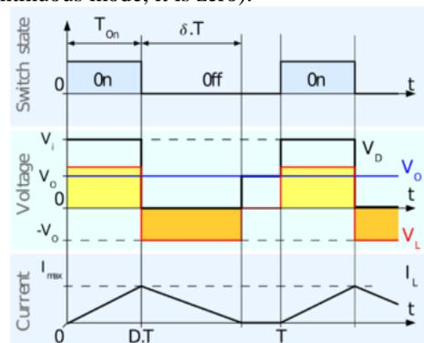
Fig.4: Evolution of the voltages and currents with time in an ideal buck converter operating in discontinuous mode.
