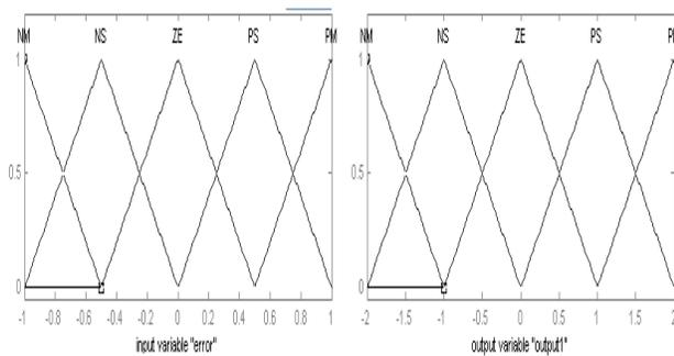
Fig.9 Triangular 5 membership functions of the error, input
