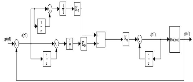
Fig.6 shows the conventional digital PD controller.
