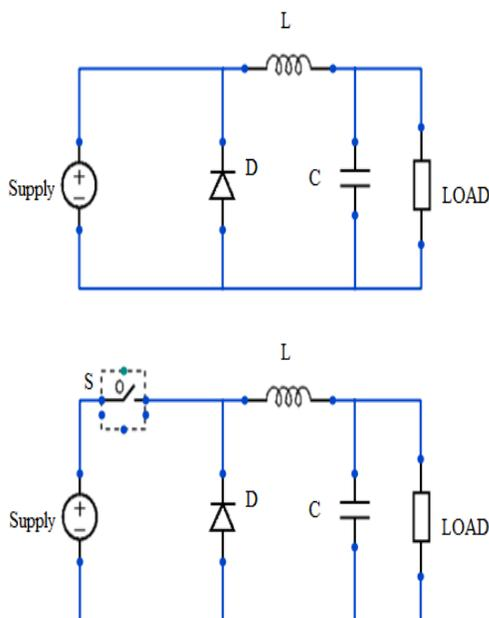
Fig.2: The two circuit configurations of a buck converter: On-state, when the switch is closed, and Off-state, when the switch is open
