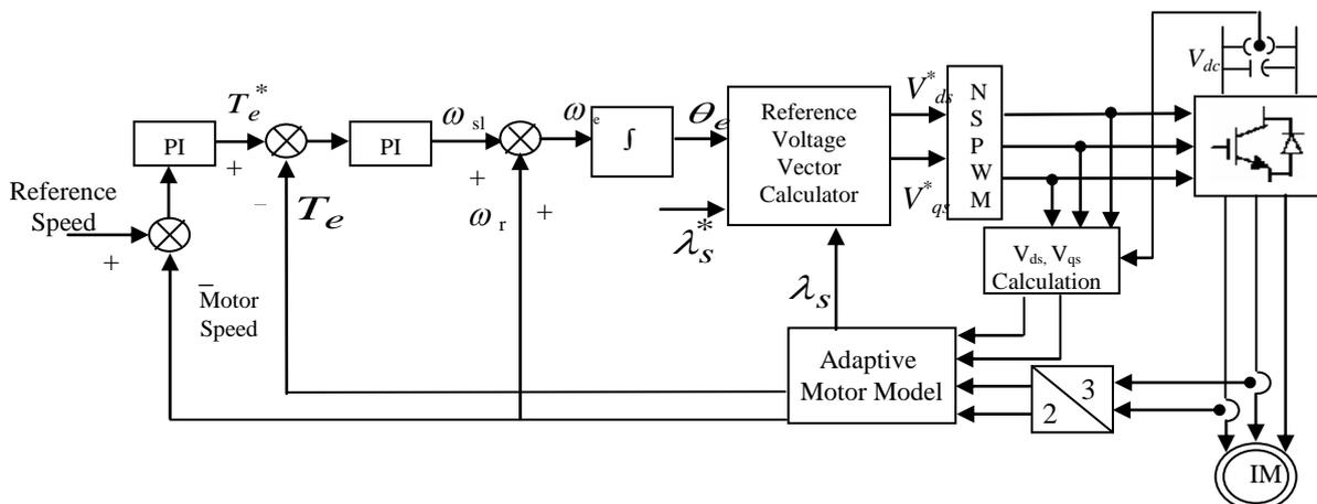
Figure 2. Block diagram of proposed PWM based DTC algorithm
