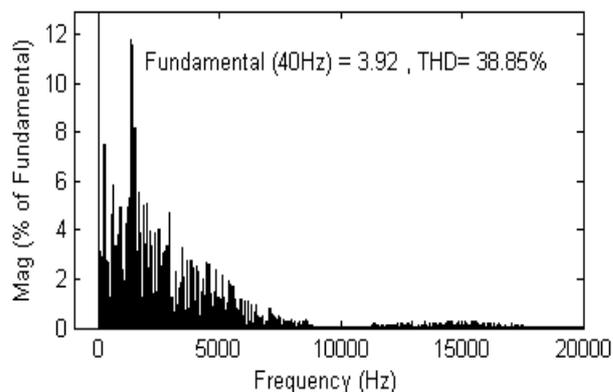
Figure 6. Total Harmonic Distortion in conventional DTC algorithm
