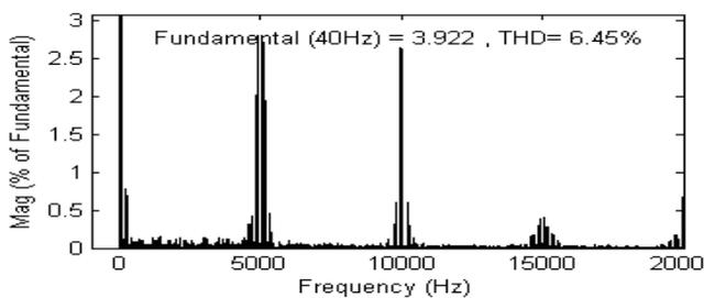
Figure 8. Total Harmonic Distortion in conventional SVPWM based DTC algorithm
