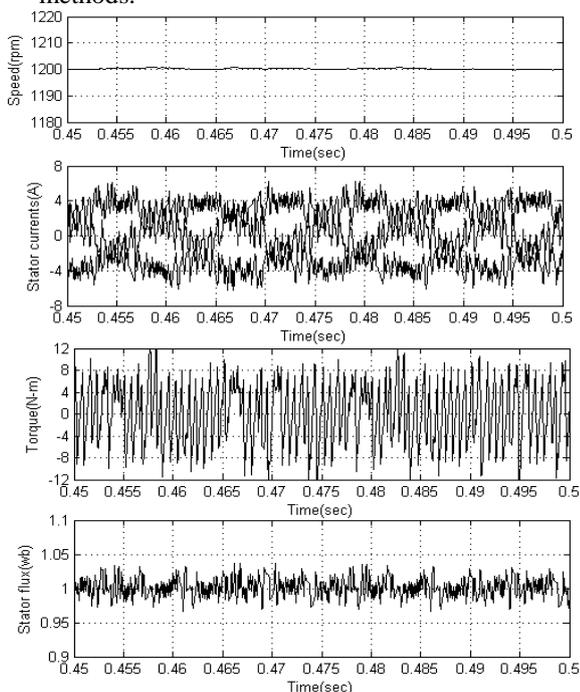
Figure 4. Steady state plots in conventional DTC algorithm
