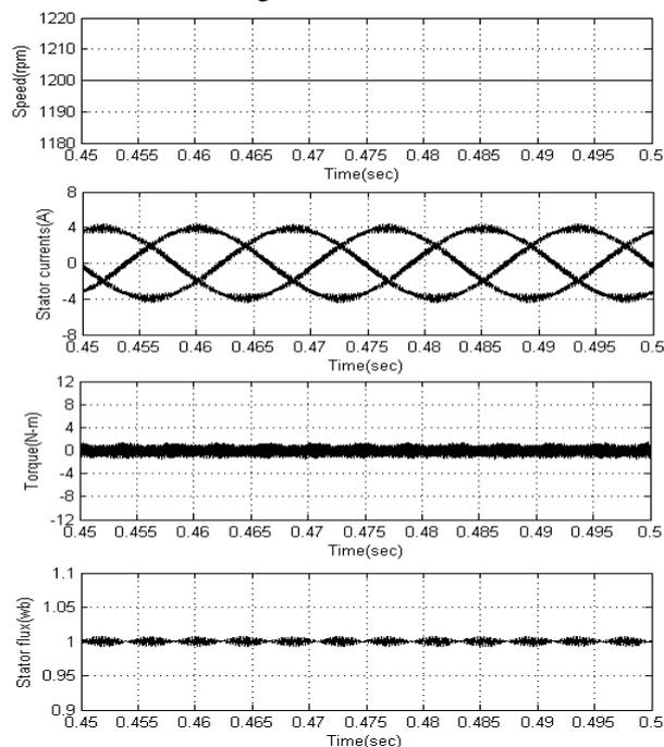
Figure 6. Steady state plots in conventional SVPWM based DTC algorithm
