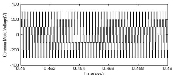
Figure 7. Common mode voltage variations in conventional SVPWM based DTC
