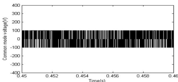
Figure 10. Common mode voltage variations in NSPWM based DTC algorithm
