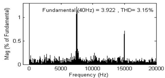
Figure 11. Total Harmonic Distortion in NSPWM based DTC algorithm
