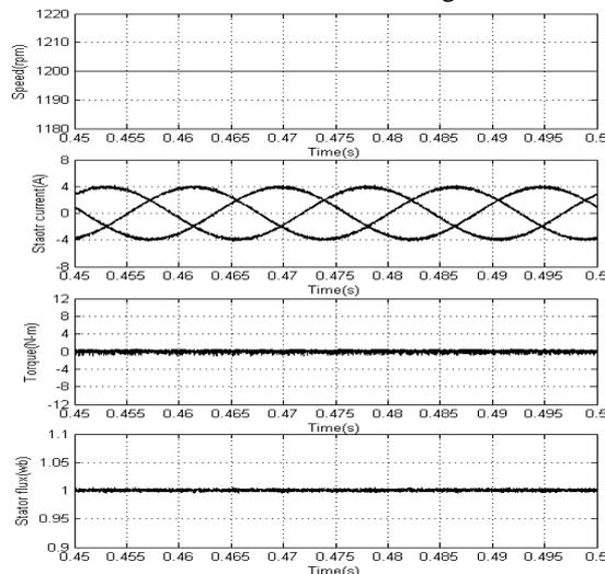
Figure 9. Steady state plots in proposed NSPWM based DTC algorithm
