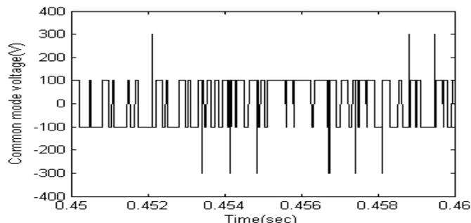
Figure 5. CMV variations in conventional DTC algorithm
