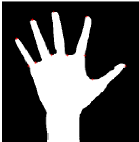
Fig 4.2 Extraction of finger tips and valley points from the segmented palm image
