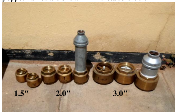
Fig. 4 shows the spring-loaded poppet valves and the corresponding extension pipes used to set the same depth of pumping of 1.75m by all the valves.
