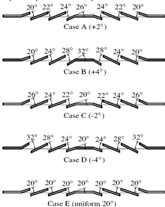
Figure 3: Different case models of heat exchanger
