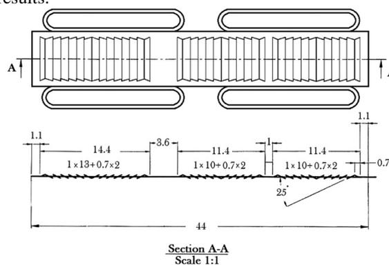
Figure 6: Asymmetrical arrangement of louvers
