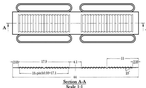
Figure 7: Symmetrical arrangement of louvers
