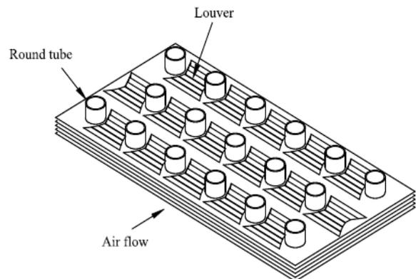
Figure 2: Circular tube louver fin pattern
