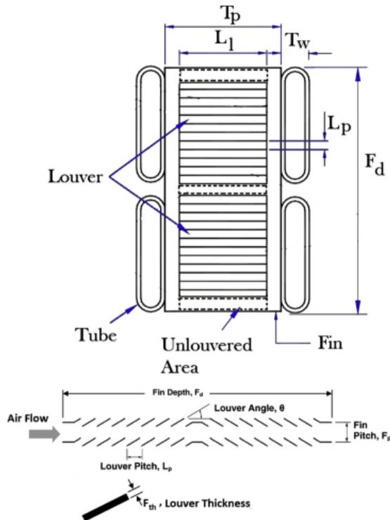
Figure 1: Typical louver fin pattern [7]
