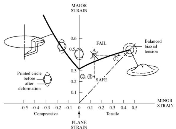
Fig.3.1 Forming limit diagram[8]
