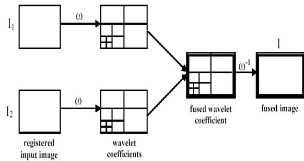
Fig 2.3 The scheme for image fusion using the wavelet transform
