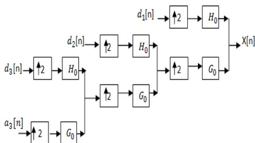
Fig 2.2 : Three-level wavelet reconstruction tree
