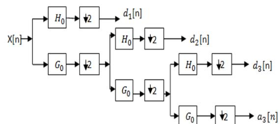
Fig 2.1 : Three-level wavelet decomposition tree
