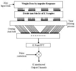
The implementation of WOLA DFT structures is as shown in the above figure where all lines represent complex data. The input sample is divided into frames of D samples and they are passed into a delay line. After they are weighted by the filter impulse response, then it is divided into blocks of K samples and overlapped to pass through the FFT. Finally the phase of the outputs is corrected.
