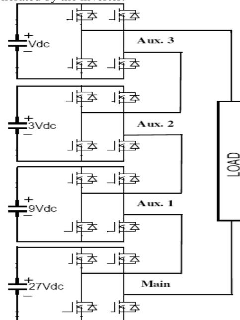
Figure.2 (a) proposed topology for 81-level inverter.
