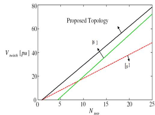
Figure.10 comparison of standing voltages on switches in the proposed topology and presented topologies in [6] and [9].
