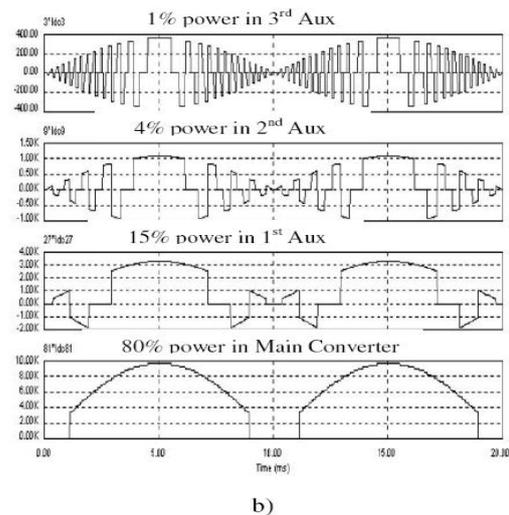
Figure.4 (b) power distribution in each converter.
