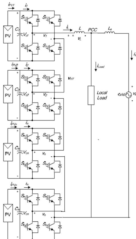
Figure.5 proposed topology for the grid-connected PV system.
