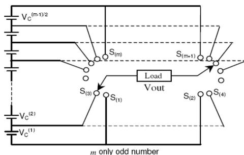
Figure.1 m-level inverter using an “H” bridge.
