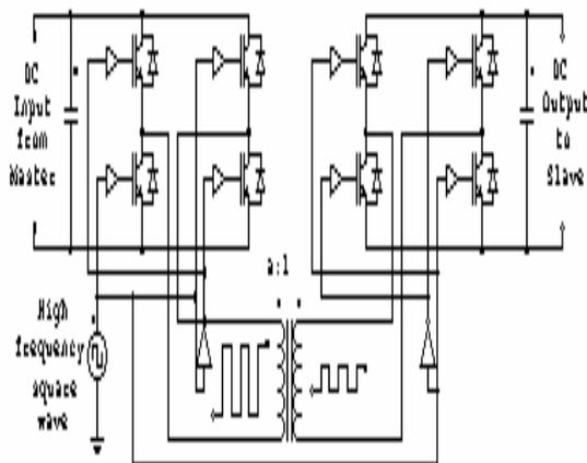
Figure.3 bidirectional DC-DC power supply
