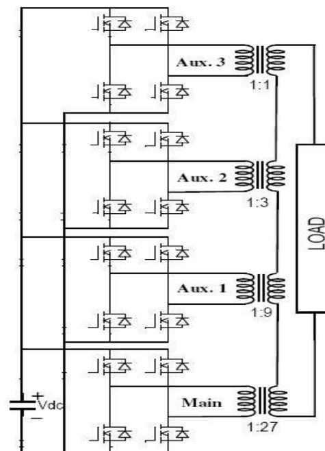
Figure.2 (b) 81-level inverter with single dc source.
