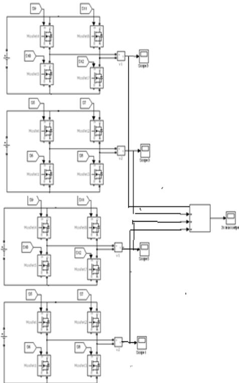
Figure.11 Matlab/Simulink model for 81-level inverter.
