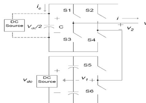
Figure.7 simplified single-phase topology of the hybrid multilevel inverter for voltage boost.
