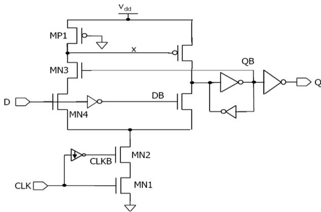
Fig.6 Single Ended Conditional Capturing Energy Recovery Flip Flop
