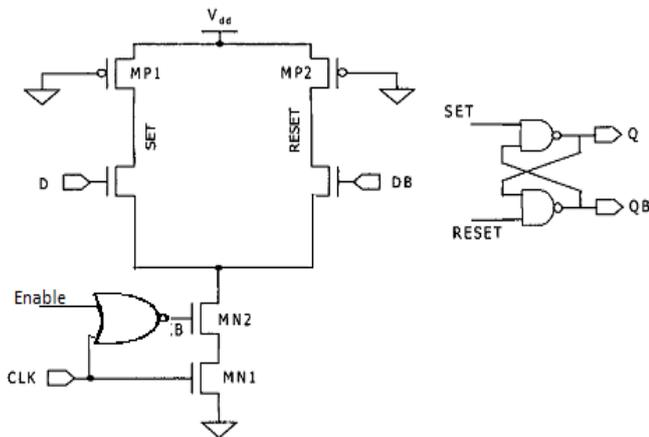
Fig.11 Proposed Clock Gating DCCER Flip Flop
