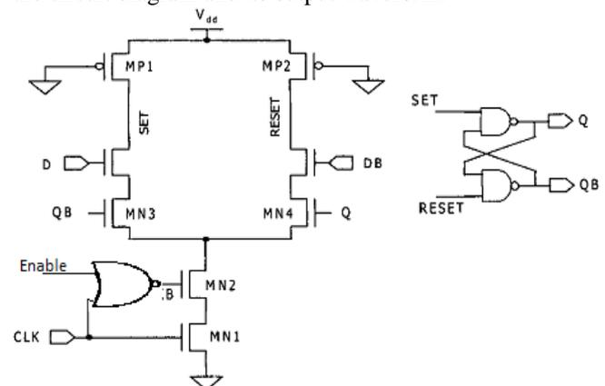
Fig.10 Clock Gating DCCER Flip Flop
