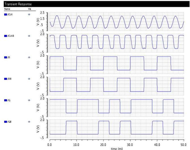
Fig. 8 the waveform of Single Ended Conditional Capturing Energy Recovery Flip Flop
