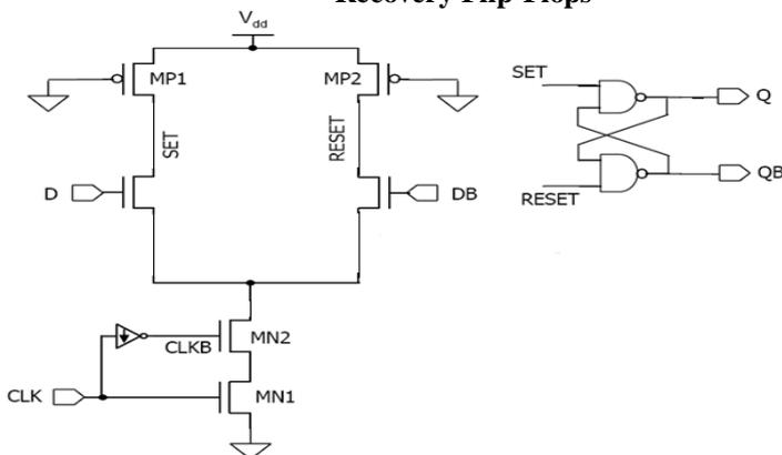
Fig.4 Proposed Differential Conditional Capturing Energy Recovery Flip Flop
