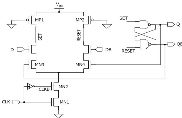
Fig.3 Differential Conditional Capturing Energy Recovery Flip Flop
