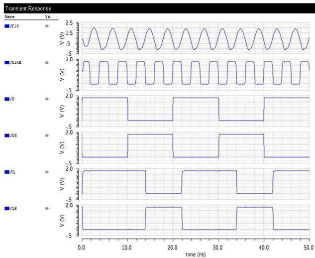
Fig.12 Waveform of Clock Gating Flip-Flops
