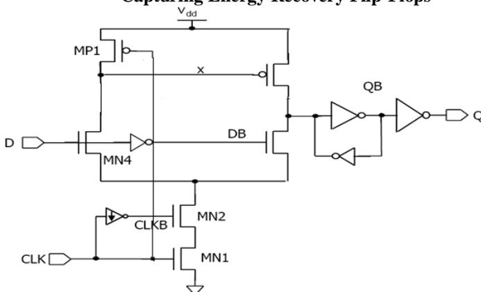
Fig. 7 Proposed of Single Ended Conditional Capturing Energy Recovery Flip Flop
