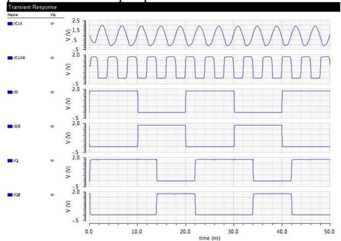
Fig.5 The output Waveform of DCCER Flip Flop
