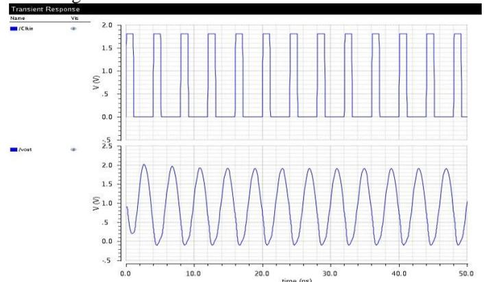
Fig. 2 Output Waveform of Energy Recovery Clock Generator
