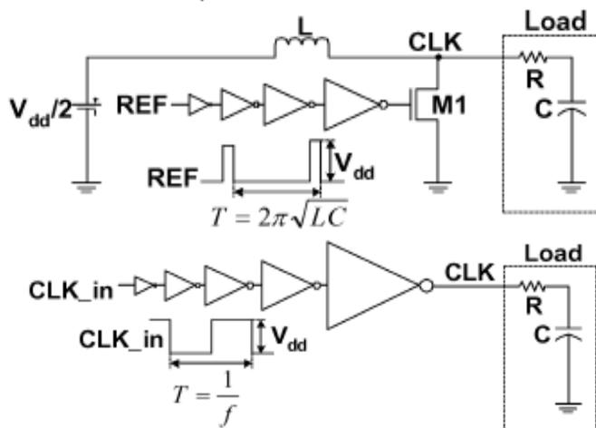
Fig 1(a): Resonant energy recovery clock generator
