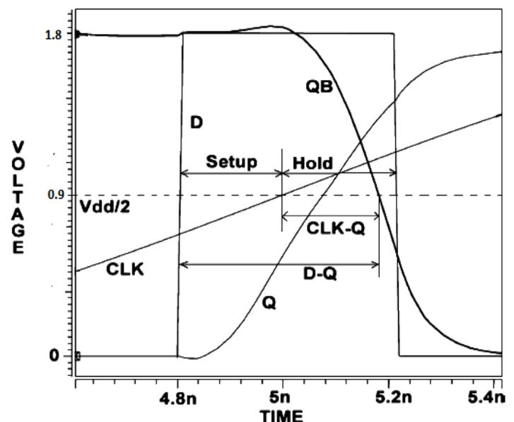
Fig. 9 Waveform of trimming definition
