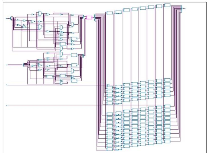
Fig.16 Pipelined Array Multiplier
