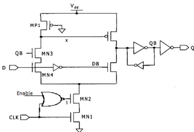
Fig. 13 Clock Gating of SCCER Flip Flop
